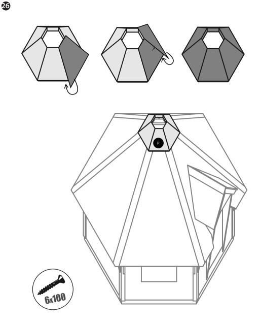
Attach the roof hat to the roof elements from below with 3 screws.
