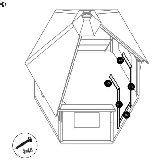
Attach door strips inside the grillhouse. The strips are attached to the door frame, wall element and roof element with 3 screws per detail.
