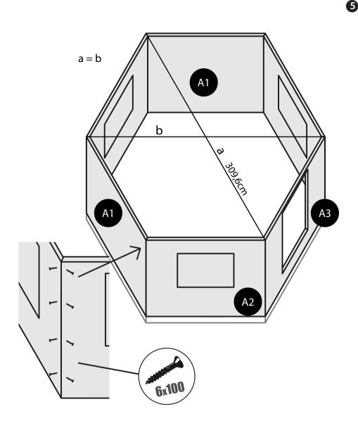
Attach the wall elements to each other using 8 screws per corner. The wall element with the openable window should be opposite to the wall element for the door.
