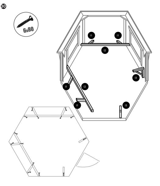
Attach the bench beams by first attaching the longer detail to the wall elements from the ends. Make sure they are parallel to the wall. Then attach the two shorter details to the previously attached detail and to the wall. Beams should be places 39cm above the floor.
