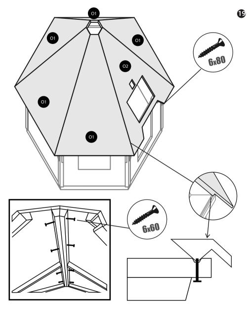
Be sure to provide support for each roof element while assembling. Use 8 screws to attach wall elements to one another and another 4 from under the brim planks. Make sure when placing the roof element with door hole (O2) that it the gaps are even to the wall element's.
