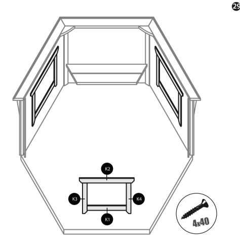
Attach the window strips inside the grillhouse. Strips are attached to the frame with ca 1.5cm overlay.
