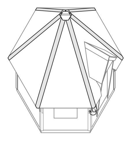
Attach peak plates to the connecting brims of the roof elements. Use felt nails. The lowest plate should be placed 7cm over the lower brim, flipped under the eaves and secured with nails.
