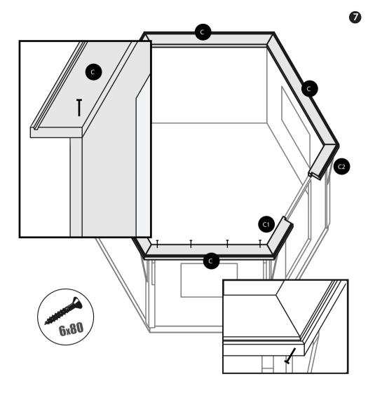
Make sure the planks inner edge is even with the walls inner side and that the corners fit nicely.
